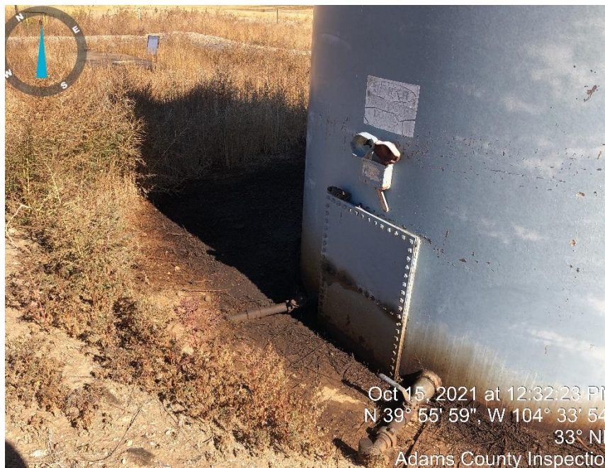
Photo #5 Stained soil around tank.
