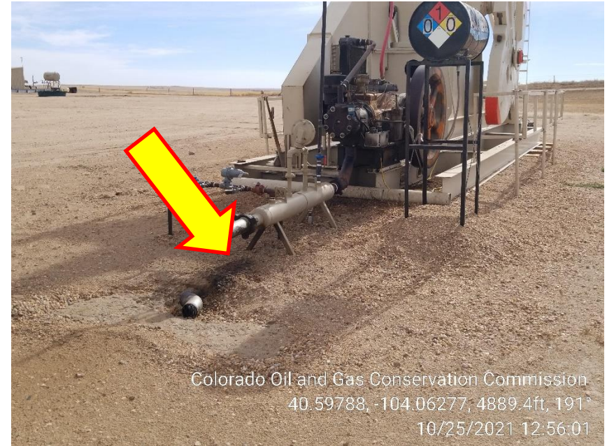
Photo 8 – Stained Soil at Exhaust
