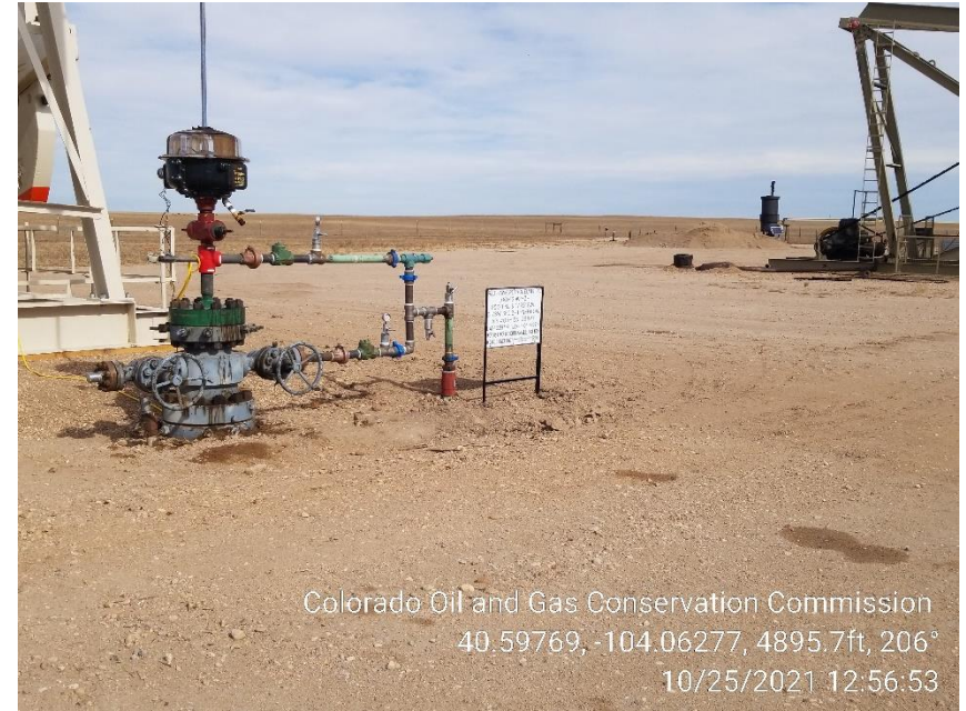
Photo 10 – Stained Soil at Wellhead
