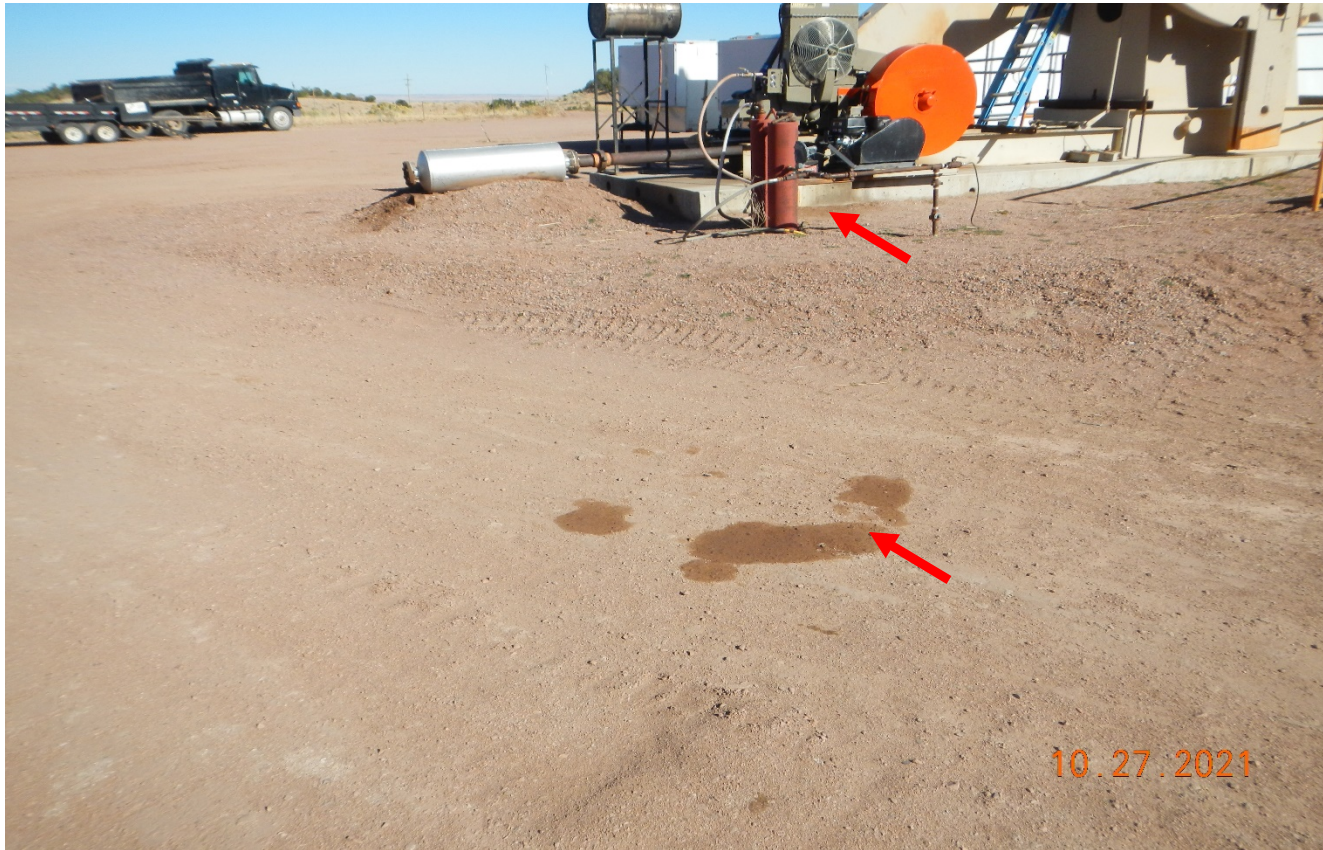
Photo 10. There is oil leaking from the pumpjack engine. There is also oil stained soil on the ground. Stained soil have not been cleaned up.
