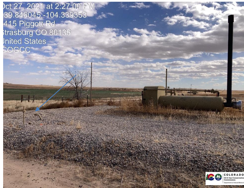
Pic 3 Separator, risers not LOTO, weeds need to be removed.
