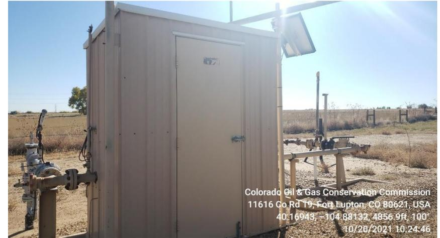
**Photo 5 Horizontal Heated Separator**
