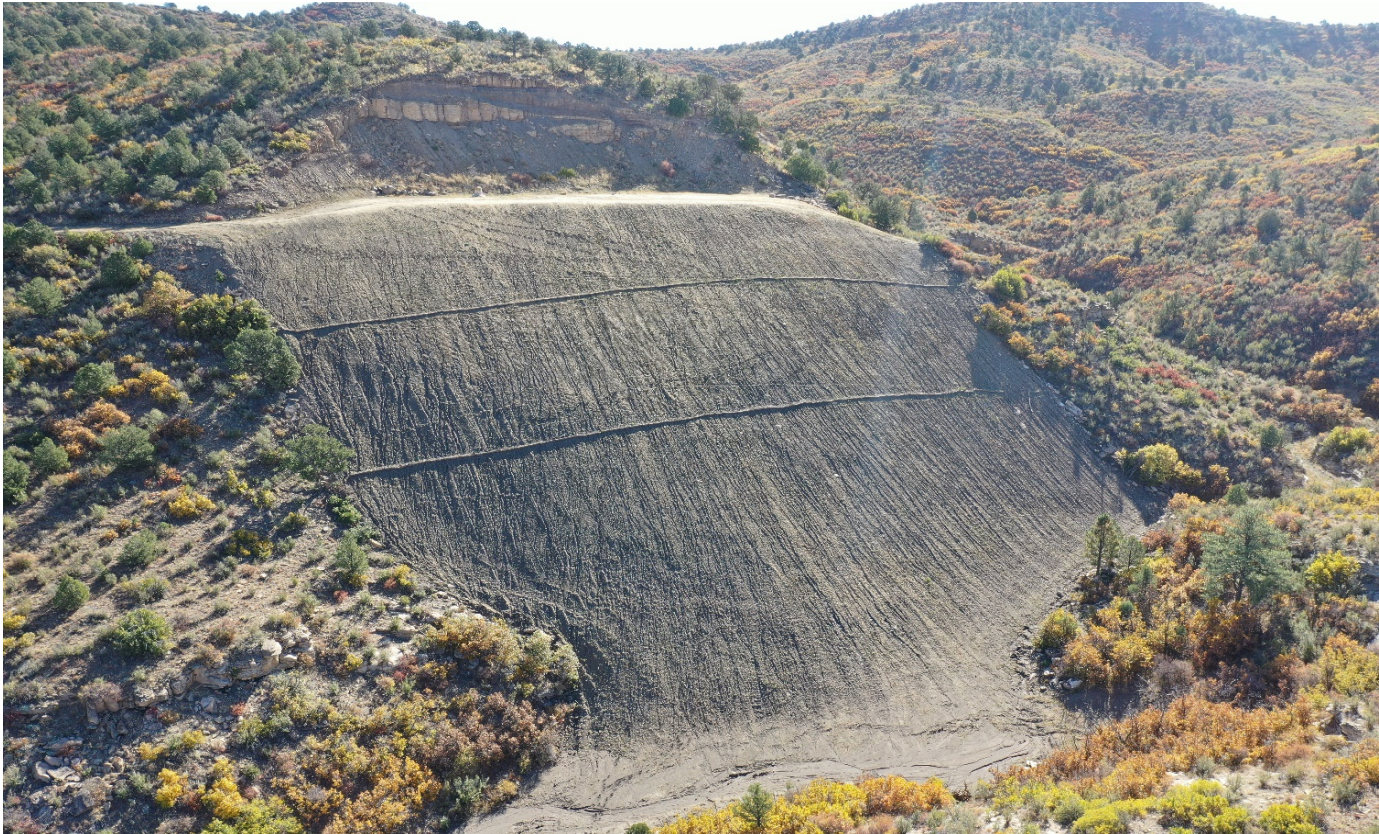
Photo 1. Drone aerial photo facing east toward the well site location. The access road and pad remain and were not recontoured back to the original condition per the rules.
