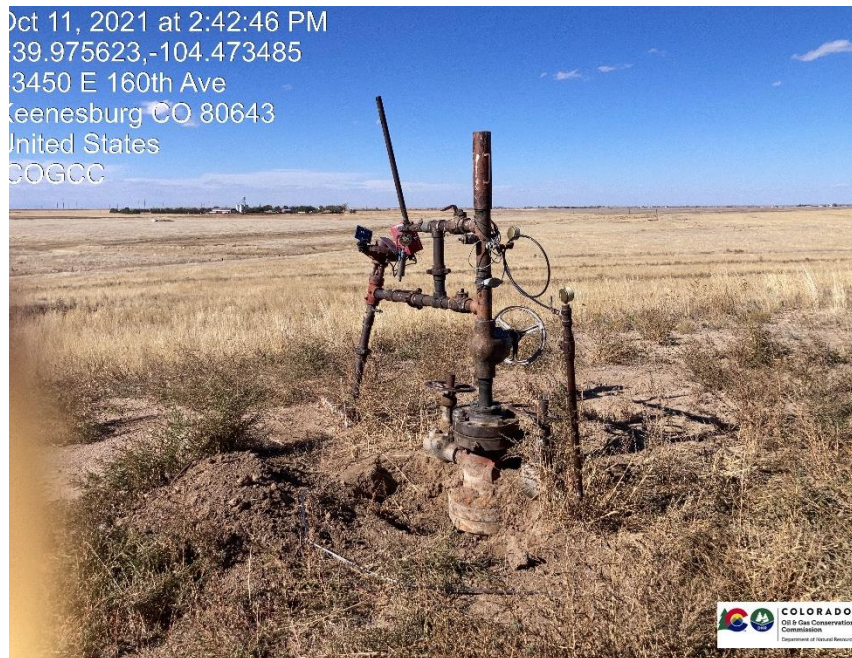
Pic 3 wellhead, bradenhead is not plumbed to surface
