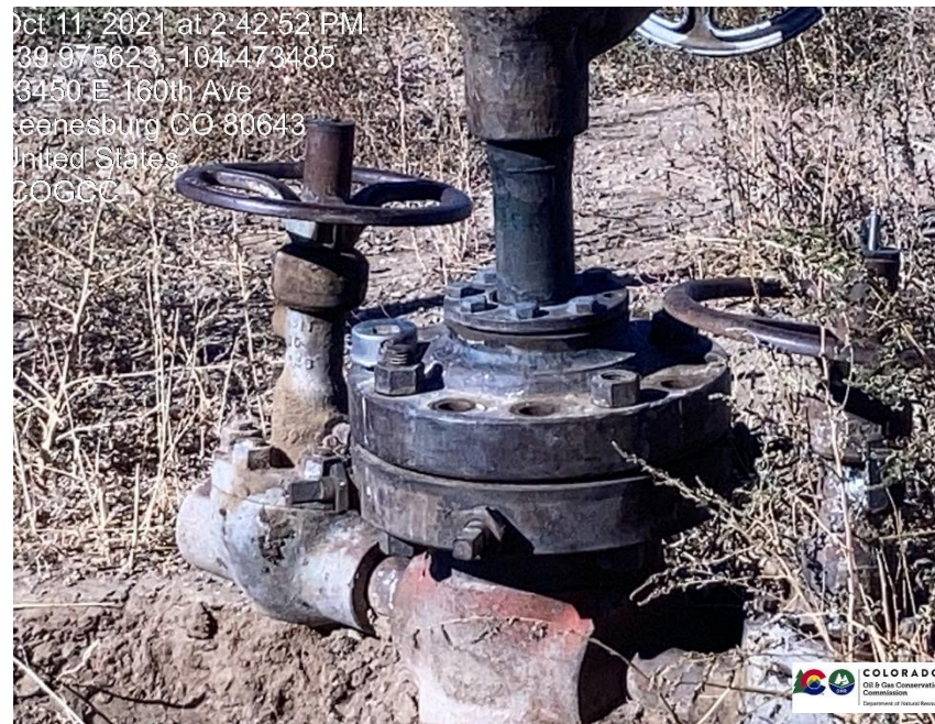
Pic 4 wellhead only has 4 bolts securing flange from wellhead to Christmas tree. Mechanical issue.
