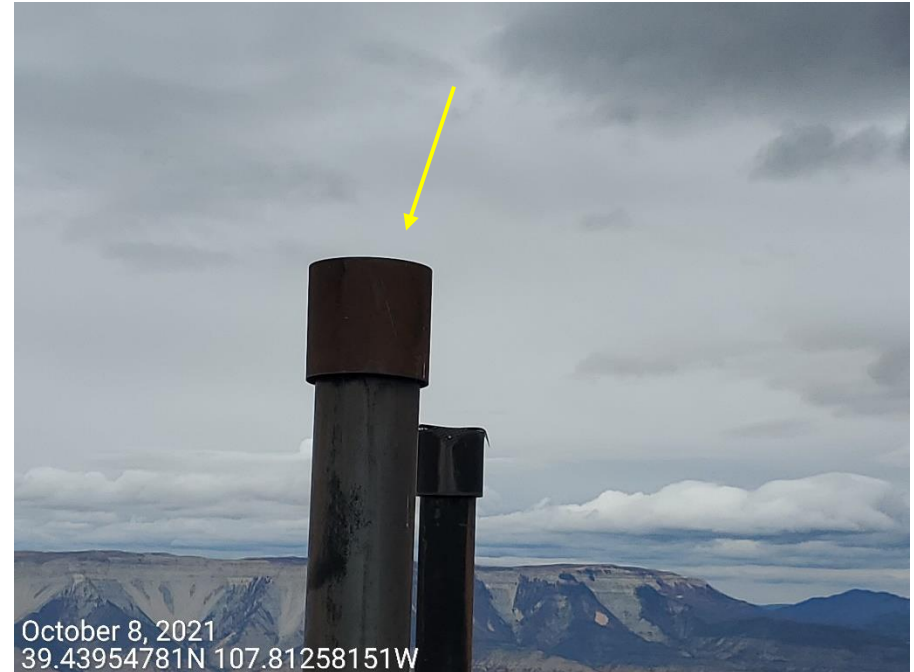
Photo 2: Photos taken from the separator equipment. Photos show wildlife protection screen has been installed on the northern separator, however, screen was not observed on the southern separator (arrow)
