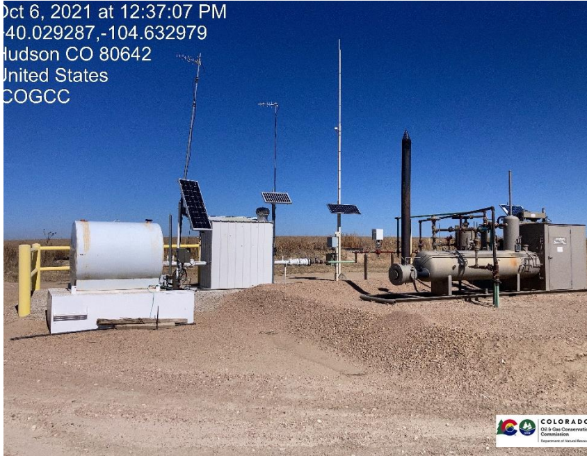
Pic 1 Separator, gas meter run, compressor, IOT automation equipment.
