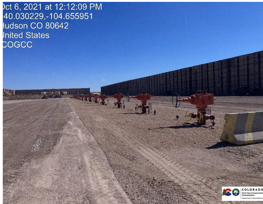
Pic 1 wellheads, prepped for stimulation with frac valve.
