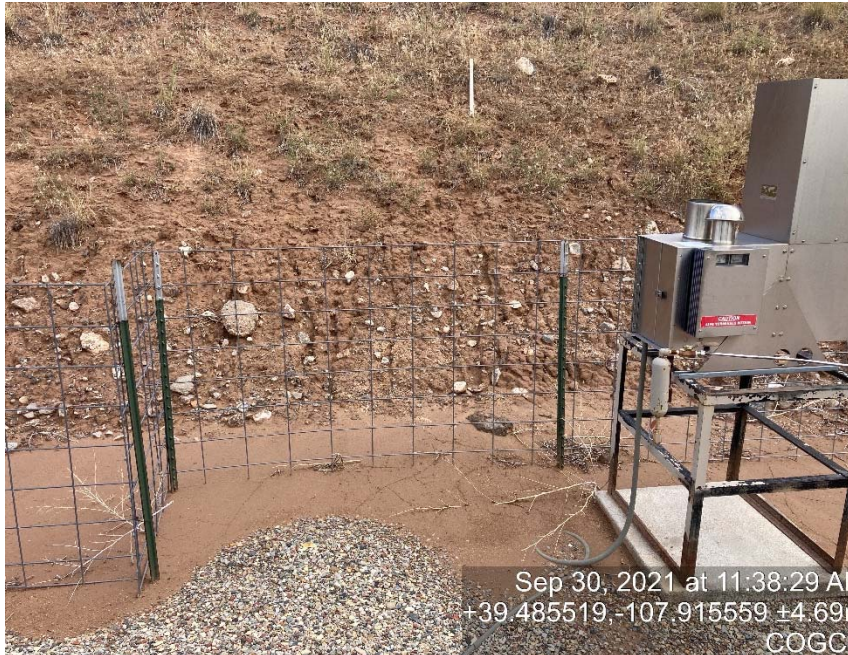
Lack of stabilization/erosion
