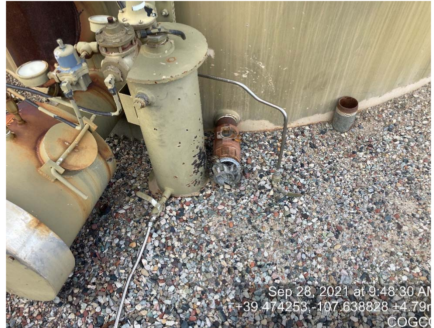
Lack of bull plug/cap and is broken
