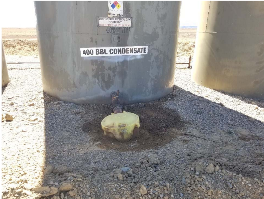
Photo 7. Stained soil at loadout.
