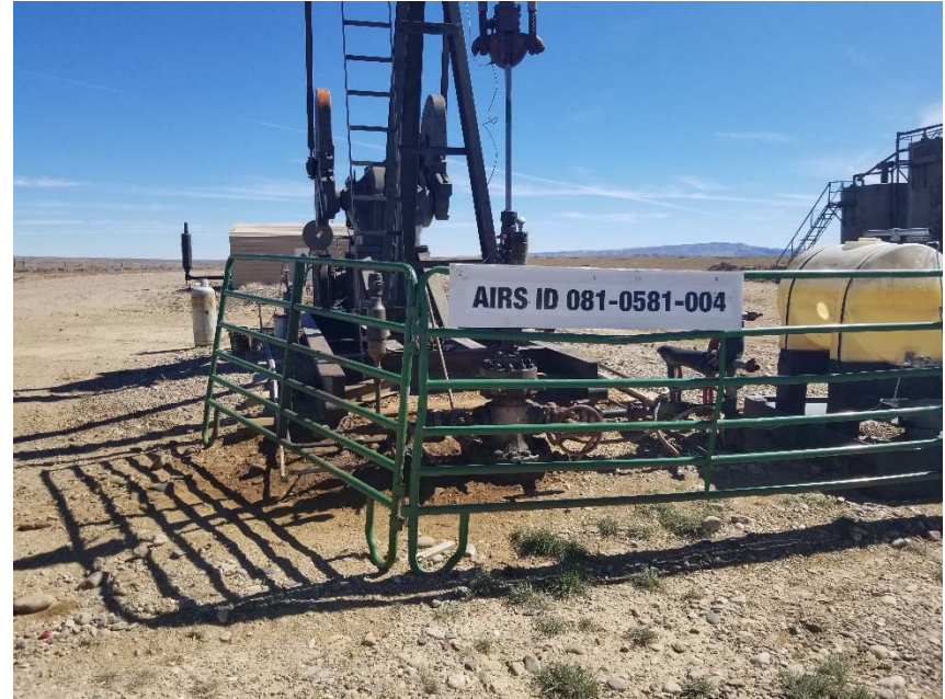
Photo 2. No wellhead sign. Stained soil at wellhead.
