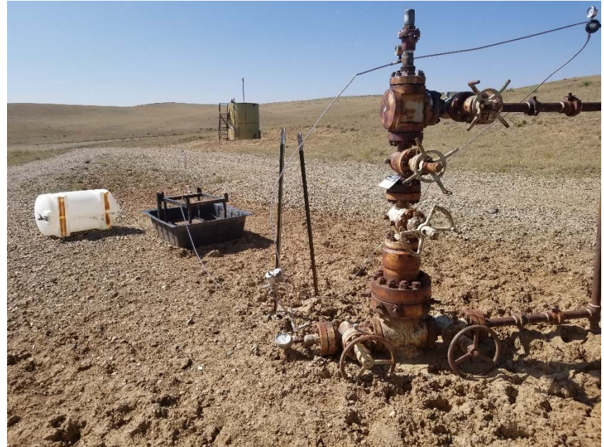
Photo 5. Tank knocked over and off secondary containment.
