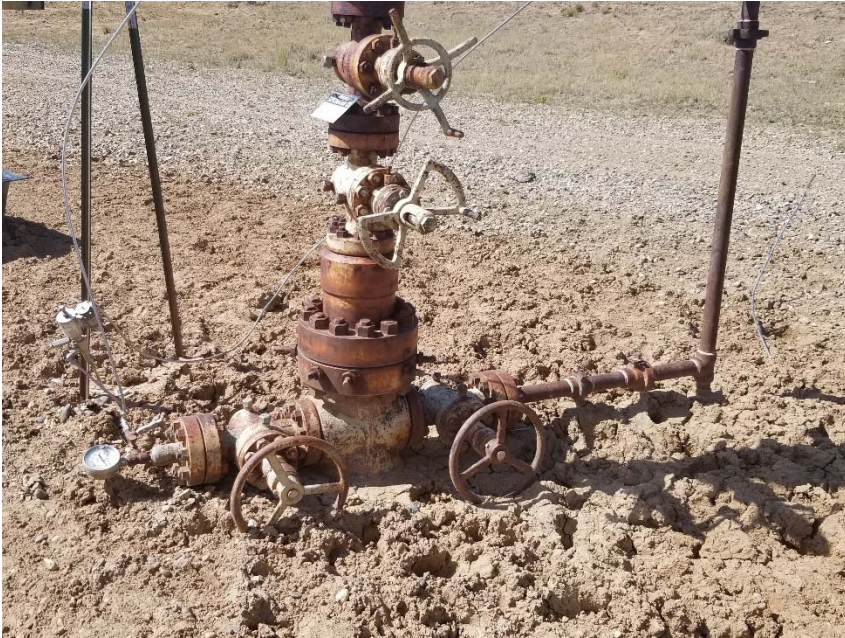
Photo 4. No bradenhead access apparent.
