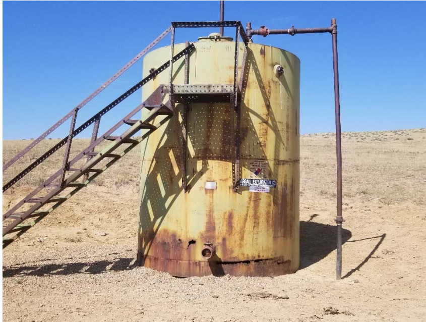
Photo 2. Tank with holes.
