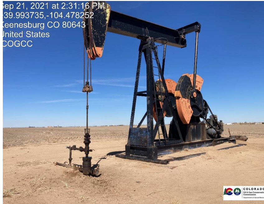
Pic 1 mechanical issue at wellhead oil is leaking on ground.
