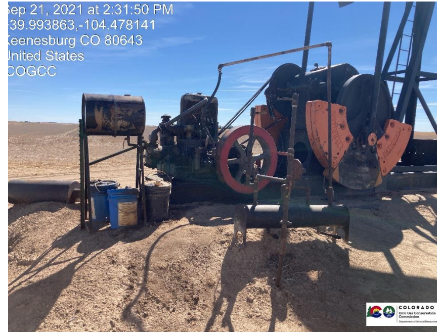
Pic 2 trash, stained soil, no containment under barrel.
