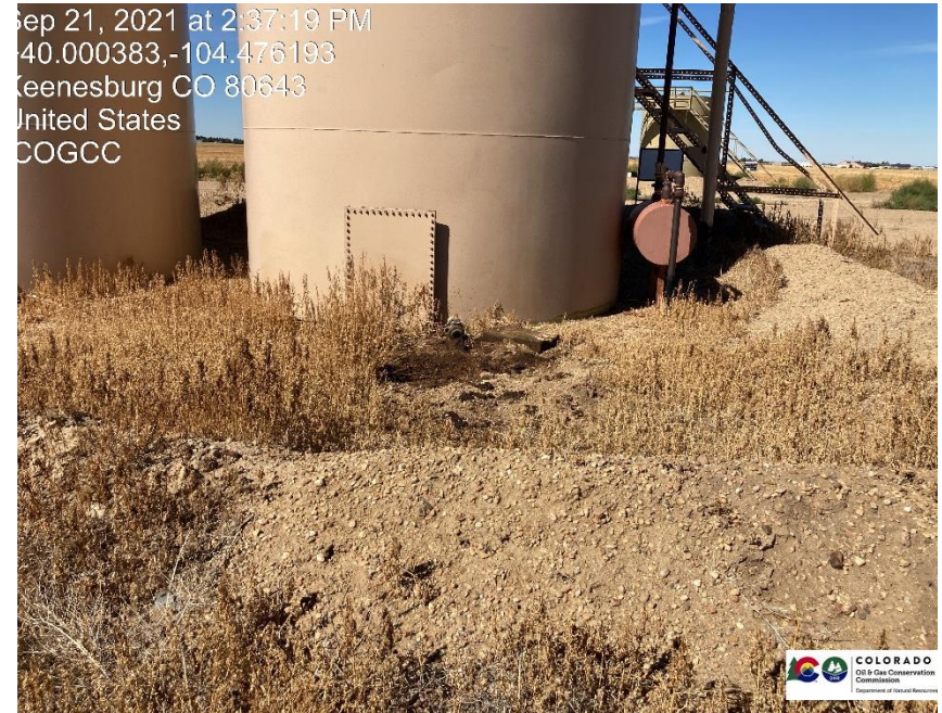
Pic 8 stained soil / mechanical issue on back of tank.
