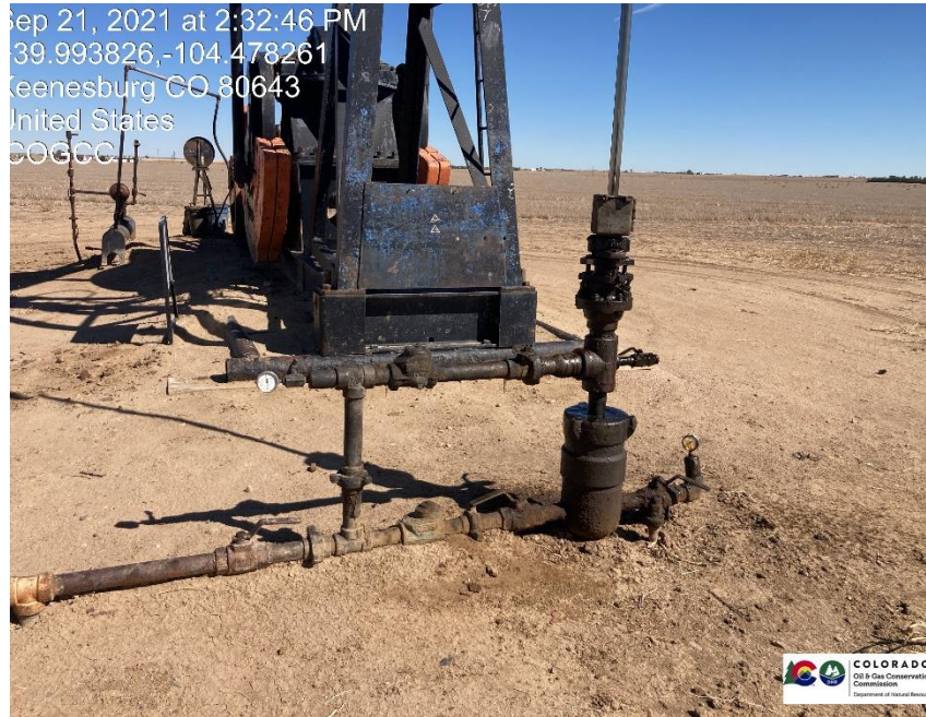
Pic 3 Stained soil/ mechanical issue by wellhead.
