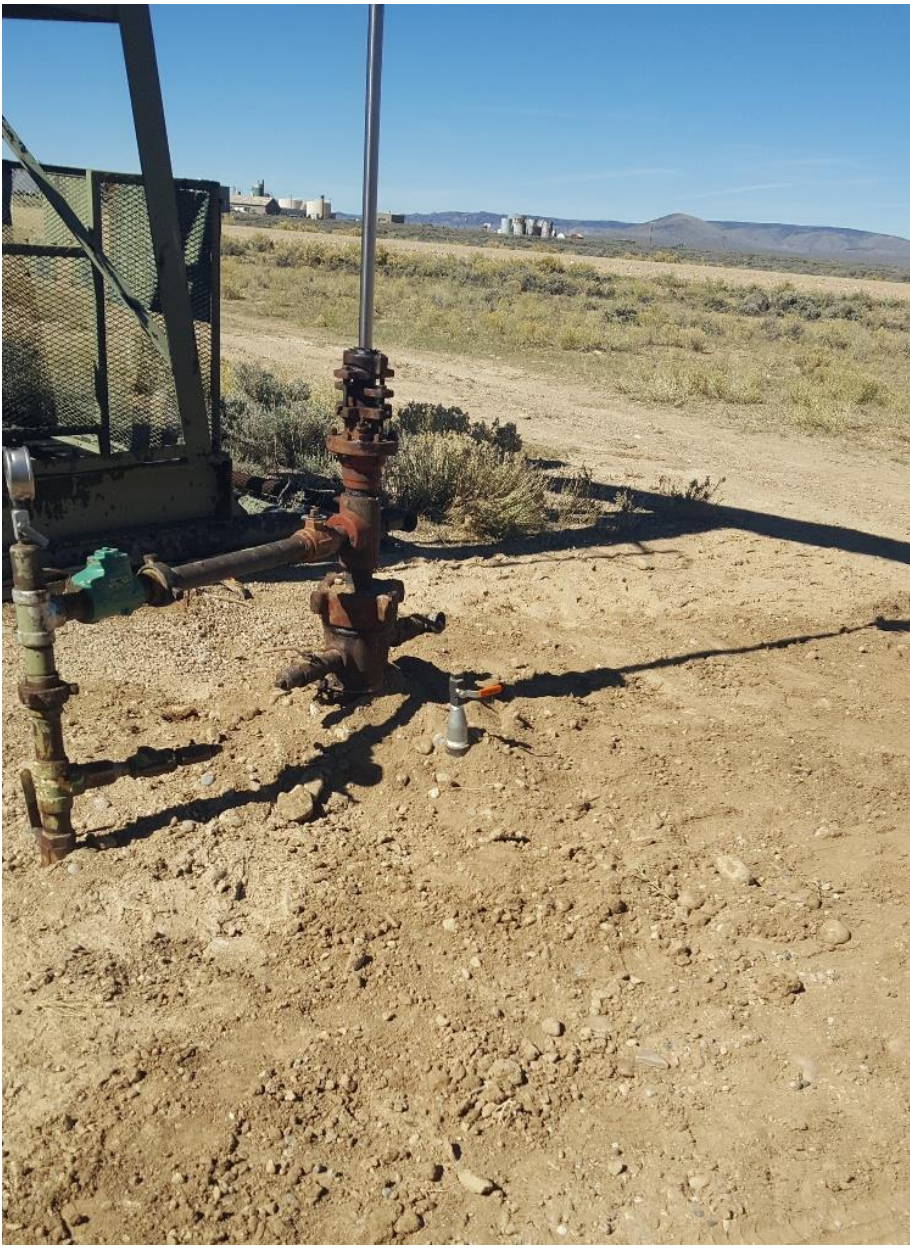
Figure #1 Bradenhead access has been installed.
