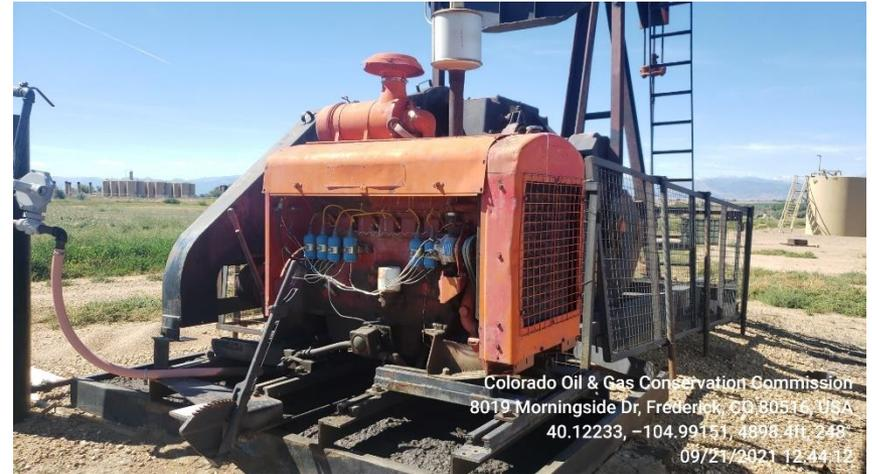
**Photo 5 Stained soil under gas engine in pump jack base**
