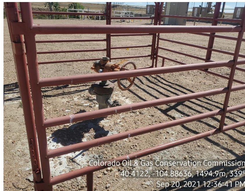
Photo 2: Wellhead (cemented)
