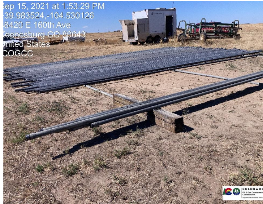
Pic 7 no containment under tubing
