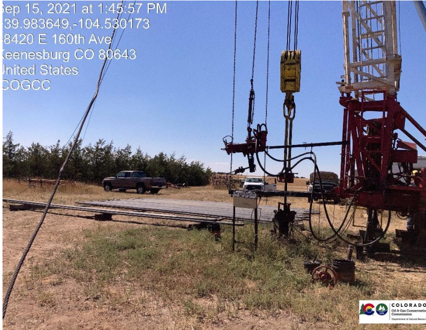
Pic 3 no Blow out preventer installed on wellhead.
