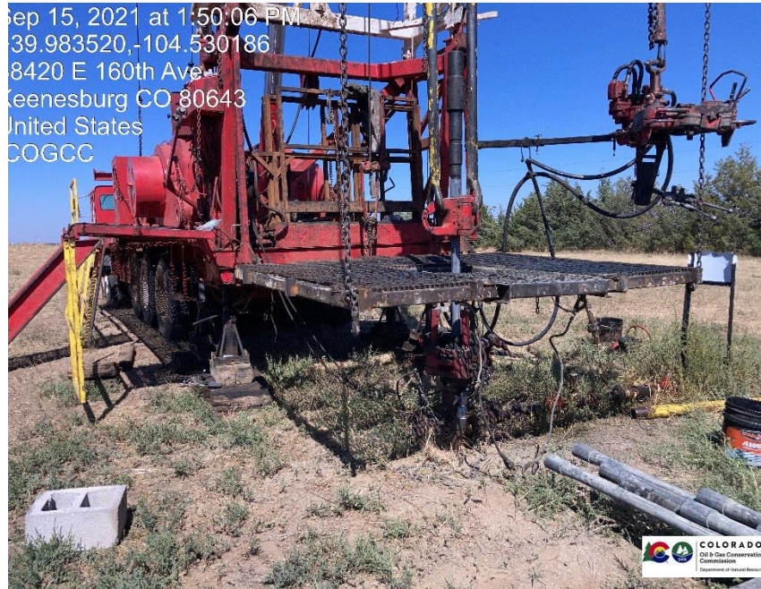
Pic 5 no blow out preventer installed on wellhead
