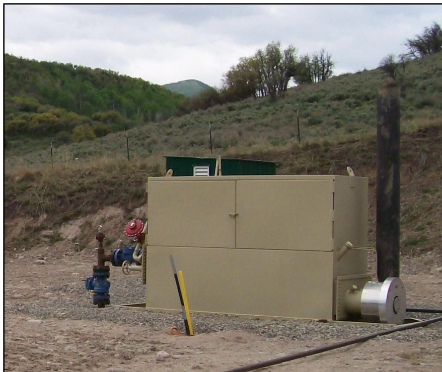
Figure 8 Gravity Separator manufactured by Valerus.
