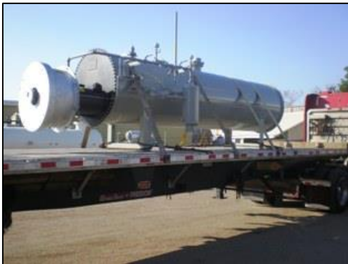
Figure 4 Line Heater from KW International
