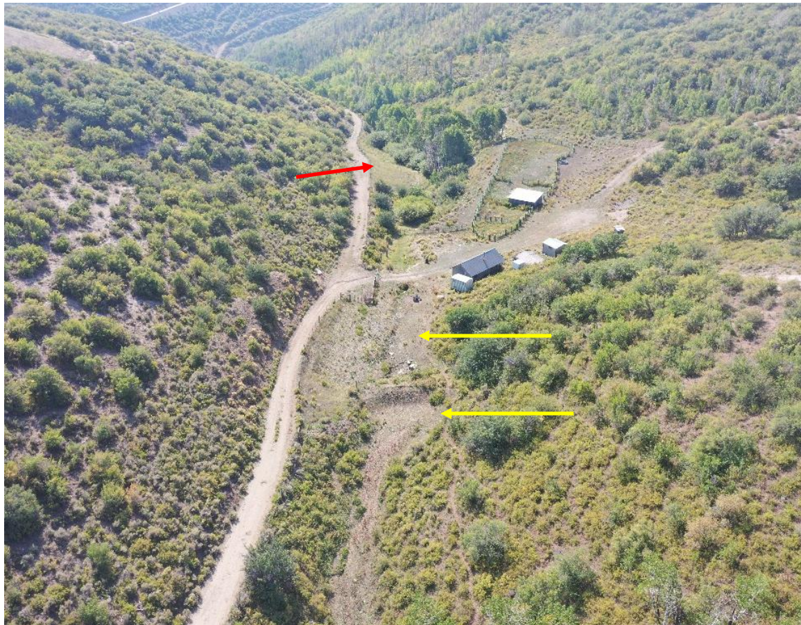
Photo 3: Aerial photo of the drainage, and Remediation Project area. Yellow arrows show disturbed areas around the “N. Trench” within Operator’s Remedial Action Workplan. Red arrow shows the area of the “S1/S2 Trench”. Upon closure of the Remediation Project, reclamation will need to be performed; Location will be required to meet 1004 reclamation standards.
