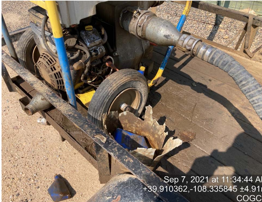
Transfer pump/debris/staining/lack of containment
