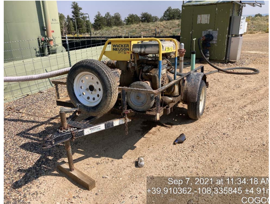
Transfer pump/debris/staining/lack of containment
