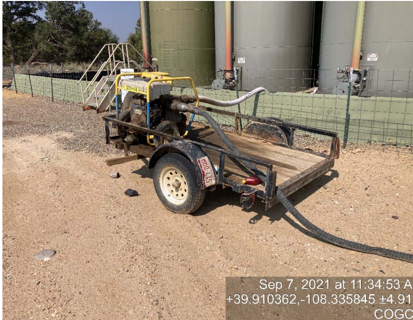
Transfer pump/debris/staining/lack of containment
