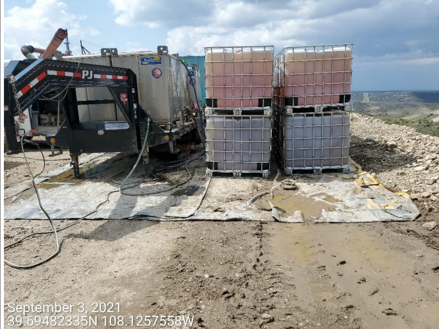
Photo 6: Photo taken from the north end of the Location. Photo shows containment BMP at tanks is not in proper functioning condition to contain a spill.
