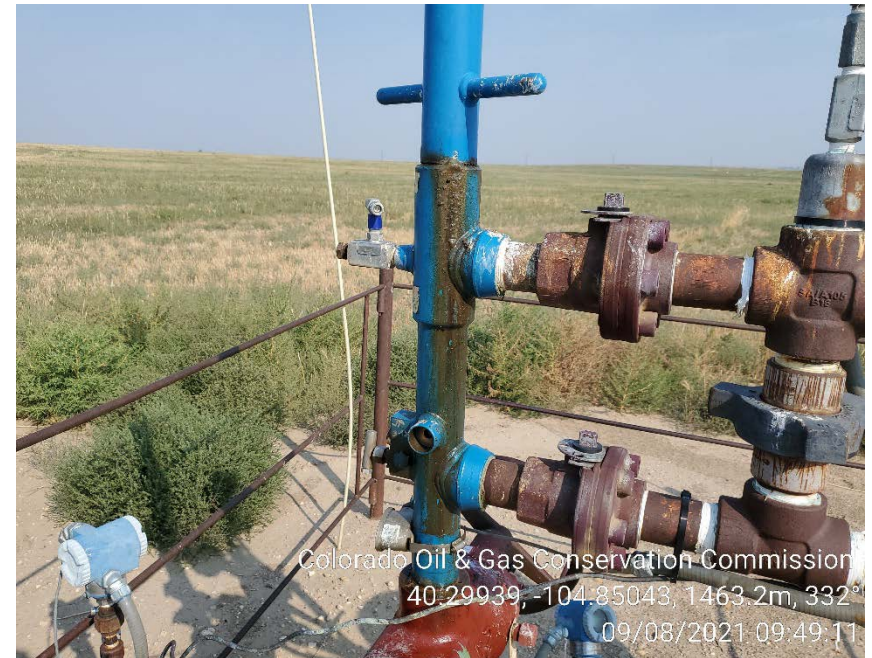
Lubricator leak
