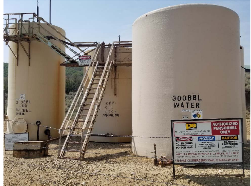
Photo 3. Some tank labels faded and no longer legible.
