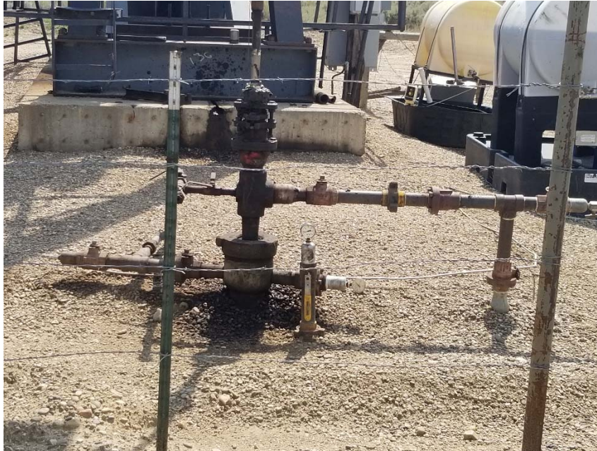
Photo 2. Stained soil at wellhead.
