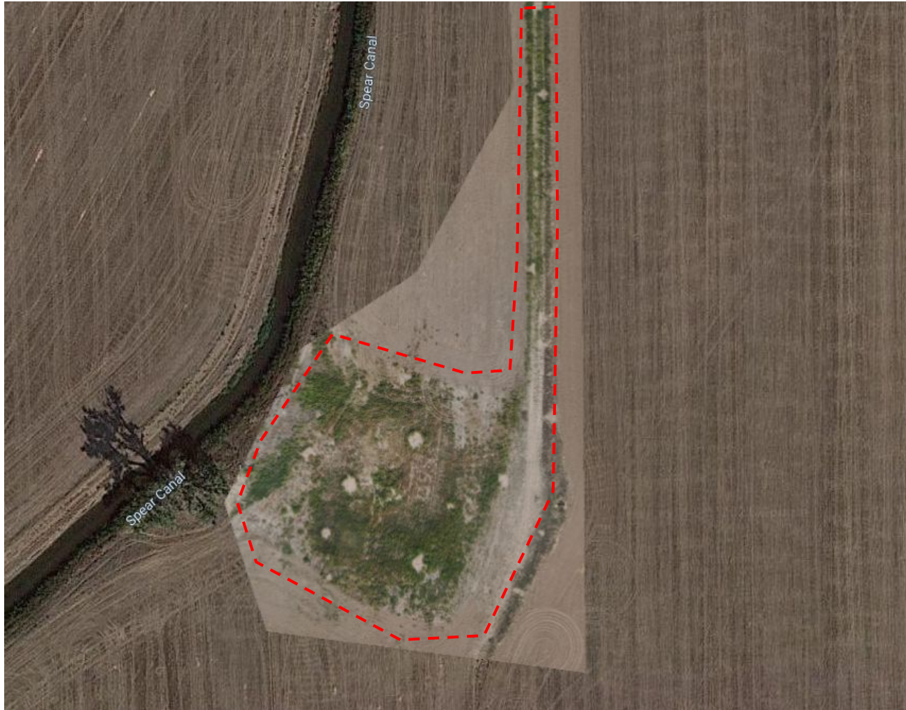
Photo 2. Drone aerial imagery of the Counter #3 well location and associated access road (red-dashed line). Operator has failed to perform final reclamation activities. Note- the access road from the Counter #2 to the Counter #3 well location has not been reclaimed and not fully pictured in the above image.
