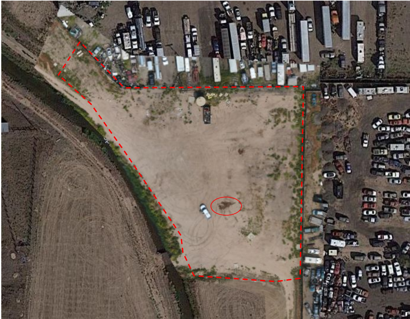
Photo 1. Drone aerial imagery of the Counter #2 well location and associated production facility (red-dashed line). Operator has failed to remove all equipment and perform final reclamation activities. Red circle is documenting a spill next to the work truck.
