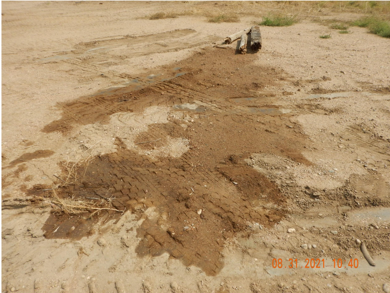
Photo 9. Photo taken from the southern production facility. Photo illustrates a spill that had smelt like hydrocarbons. Spill was approximately the size of a work truck- see Photo 1.
