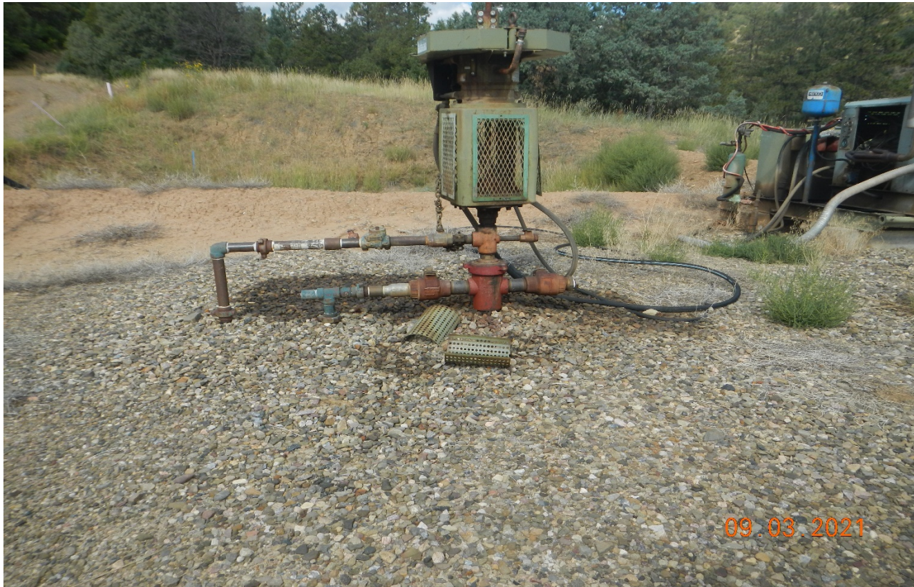
Photo 6. There is stained gravel around the wellhead indicating a previous leak. This area needs to be cleaned up.
