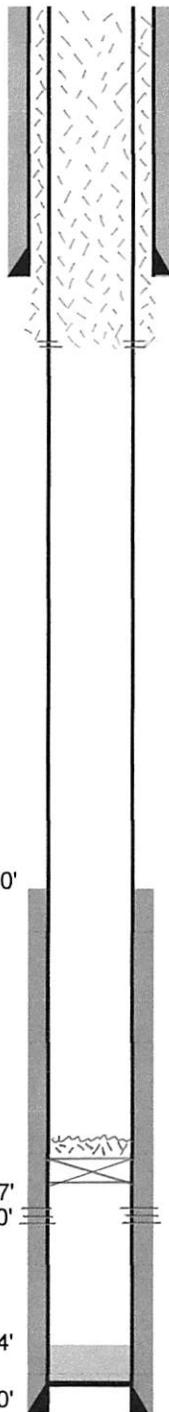
4.5" casing and 4.5" x 7" casing annulus cemented from 0'- 485' with 95 sacks 15.8#/gal class G cement. Yield is 1.15
