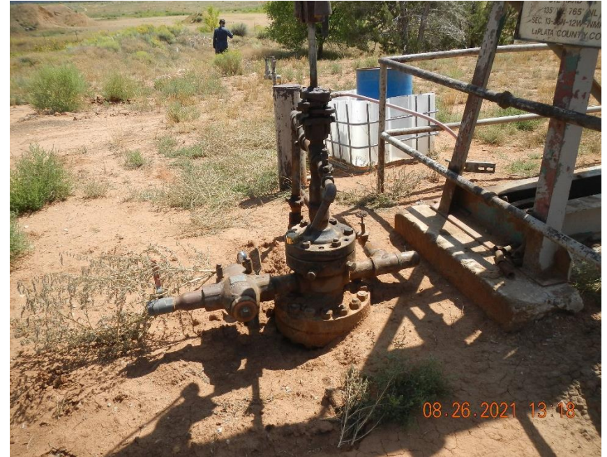
Dye Hard #1 well head.
