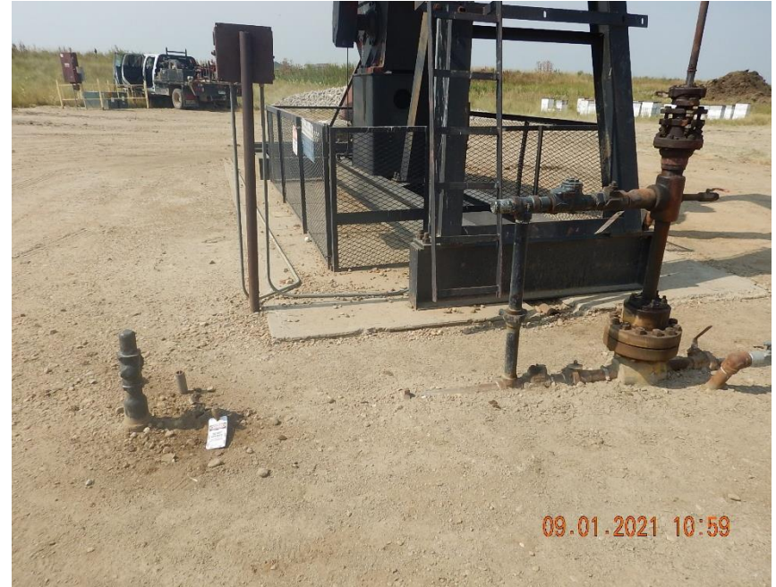
Martin J Schaefer #2 wellhead; flowline valves SI/ OOSLAT
