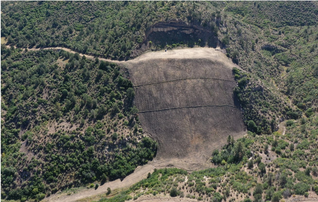
Photo 1. Drone aerial photo facing east toward the well site location. The access road and pad remain and were not recontoured back to the original condition per the rules.
