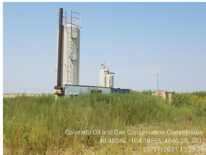
Photo 4 – Heater Treater – WEEDS
