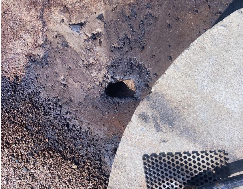
Pic 3 possible underground leak from flowline
