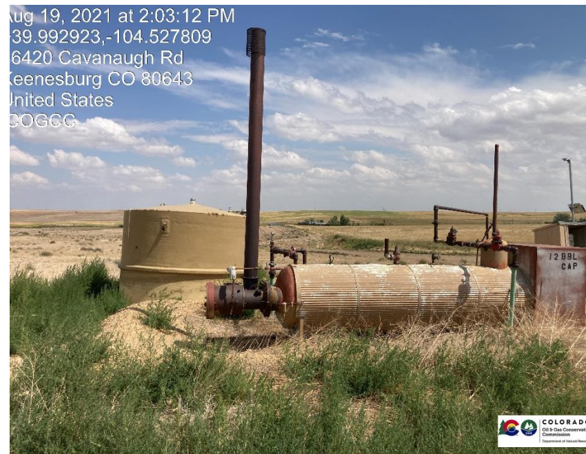
Pic 2 separator, gas meter run, unused tank on location
