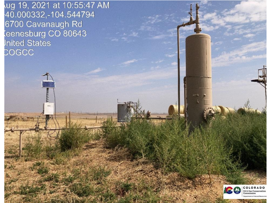
Pic 2 separator, gas meter run, weeds unmanaged
