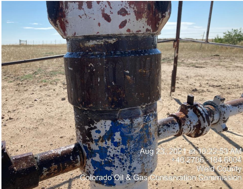
Photo #3 Leaking casing nut on threads
