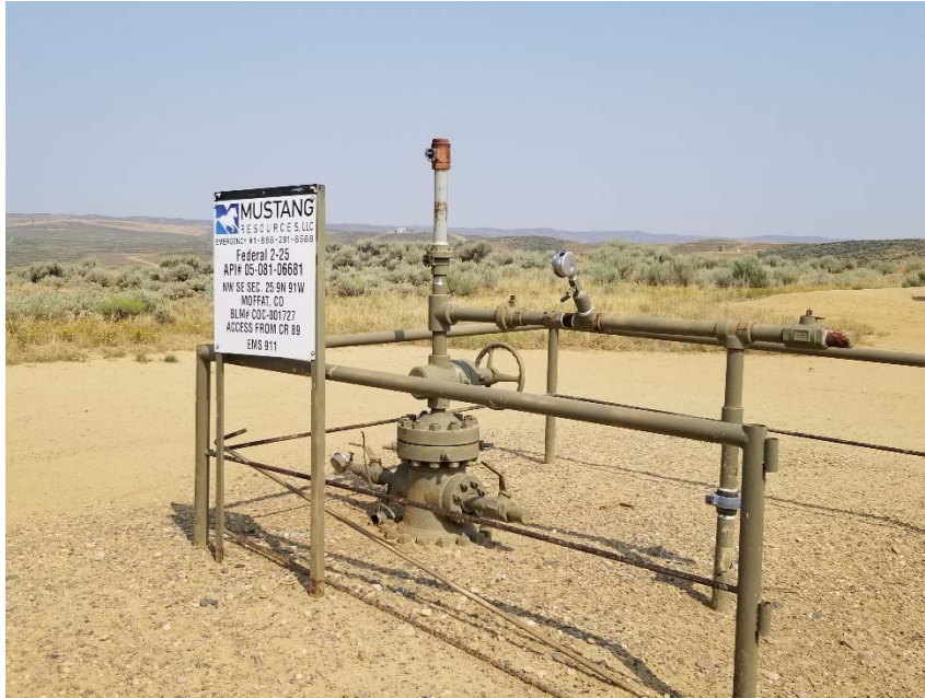
Photo 2. Signs still have previous operator information. No bradenhead access apparent.
