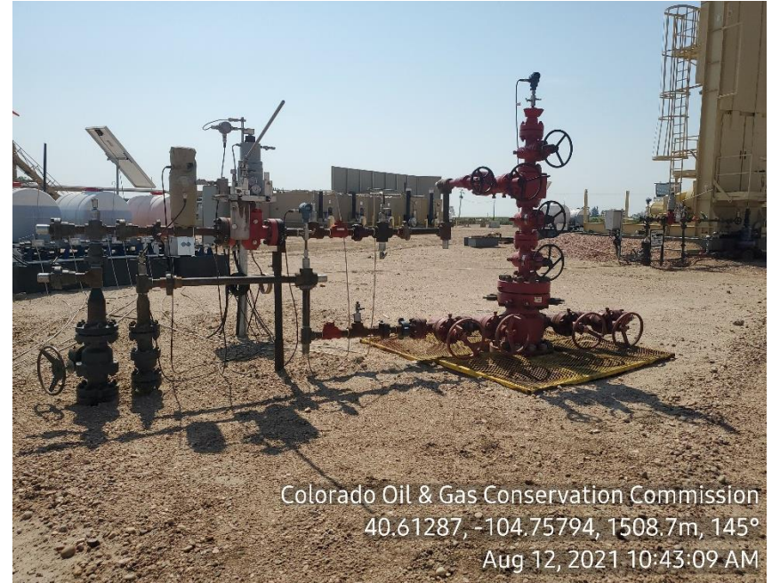
Photo 6: Wellhead does not display signage
