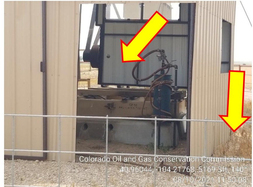
Photo 2 – Gas Engine has been removed
