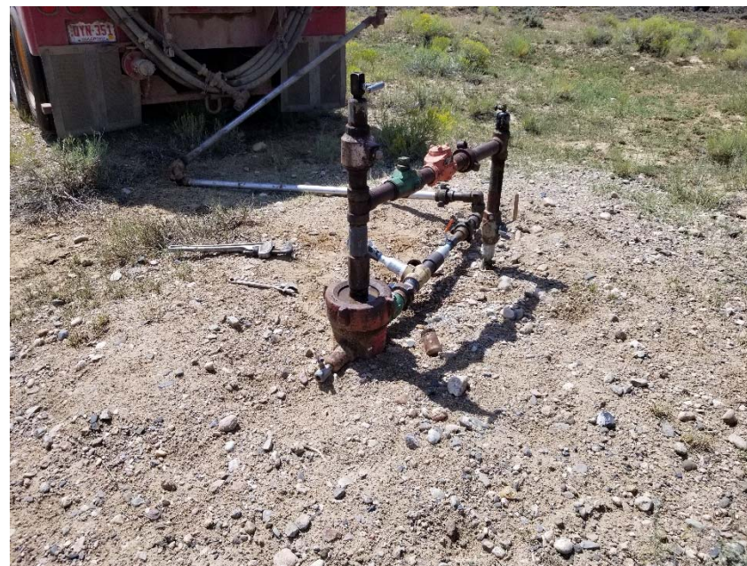
Photo 2. No bradenhead access apparent.
