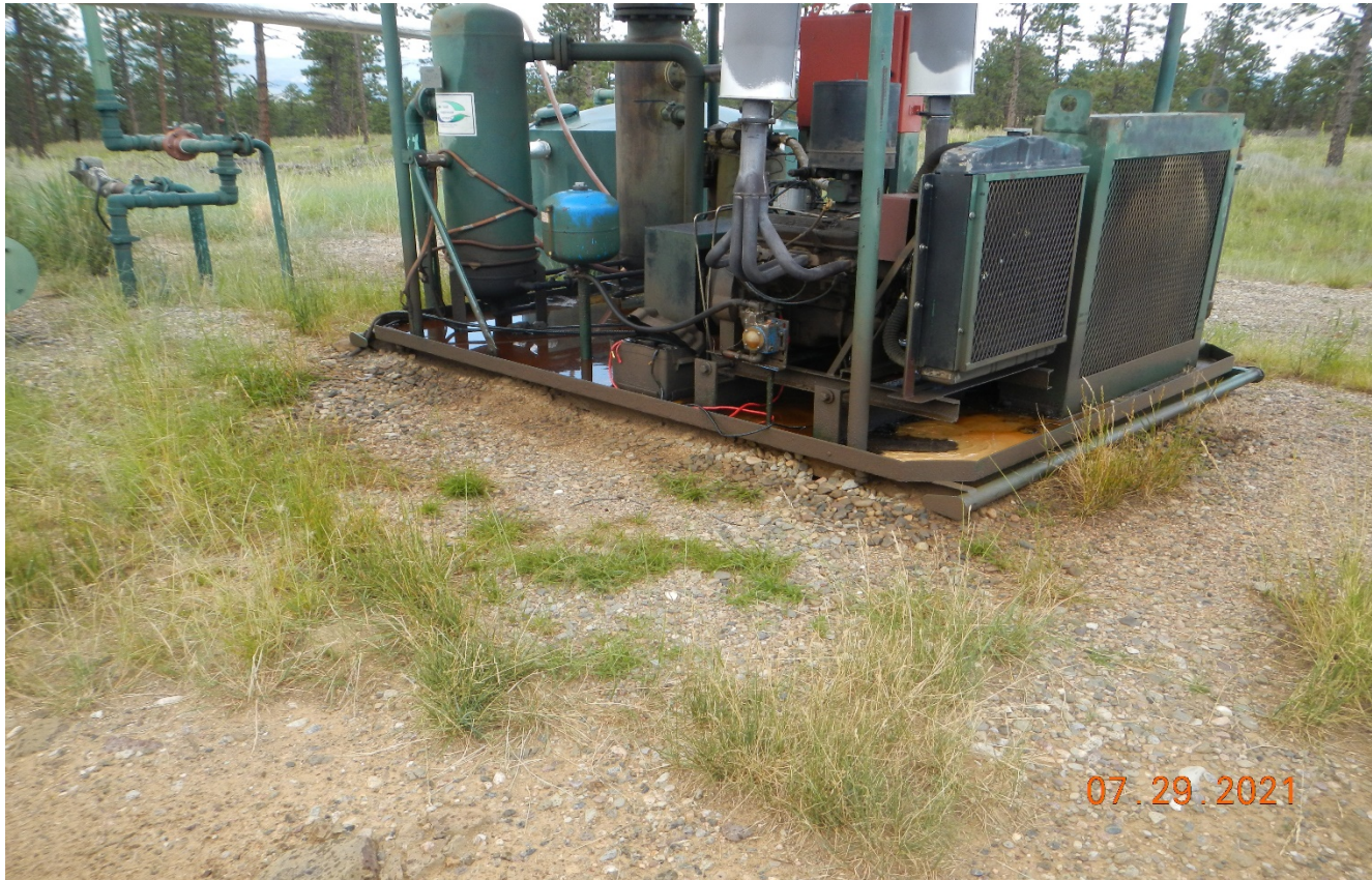
Photo 4. There is still oil inside the engine skid that needs to be cleaned up.
