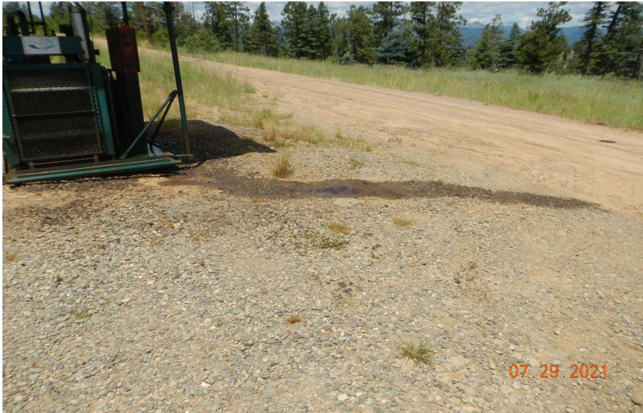
Photo 3. There was an oil leak at the engine causing oil to spill across the ground.
