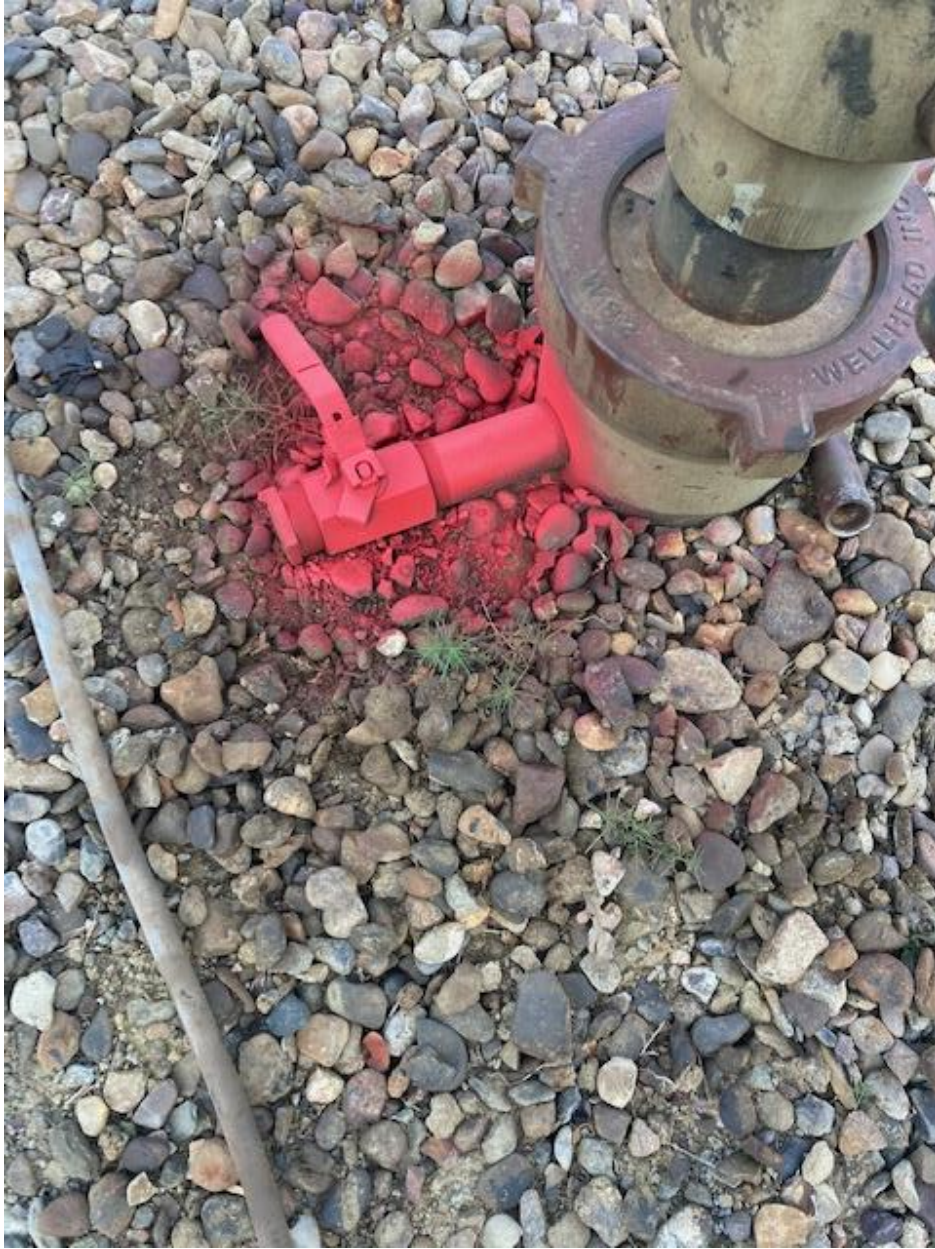
Installed appropriate fittings to allow bradenhead visual inspection as per Rule 419.a.(1), (2).
