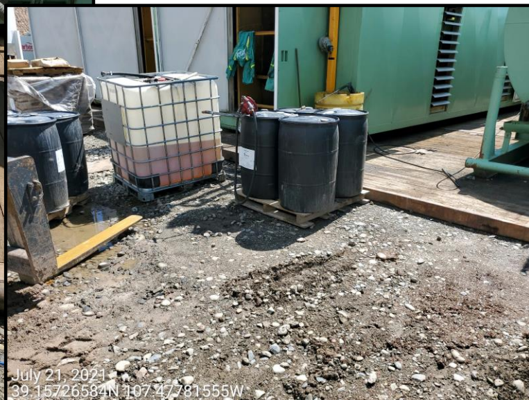
Photo 15: Photo shows example of barrels/tanks/containers observed stored on the location without proper secondary containment; BMPs missing or insufficient to contain spill.
