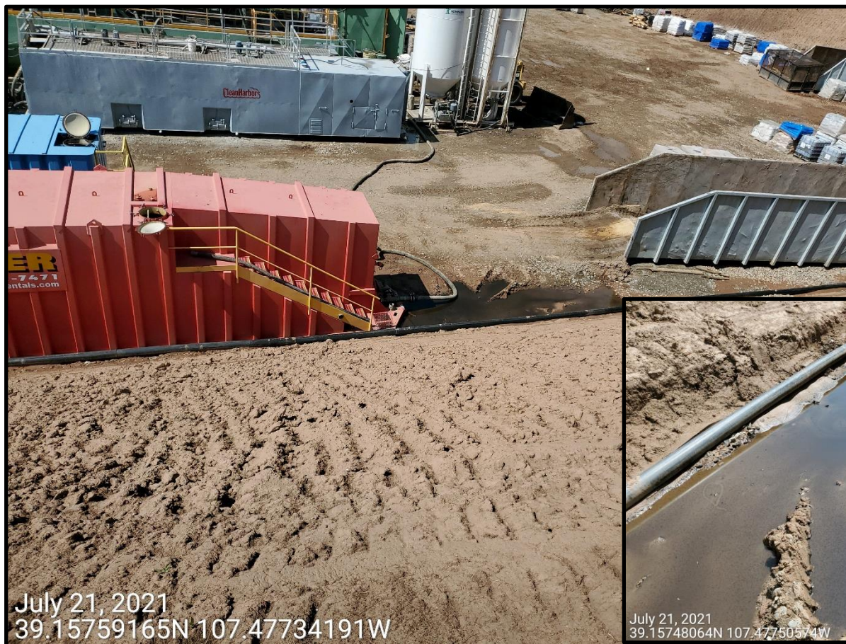
Photo 18: Photo taken from the east end of the Location, facing west. Photos 18-21 provide example of various spills and impacted stormwater observed on the Location, including within the perimeter stormwater ditch.
