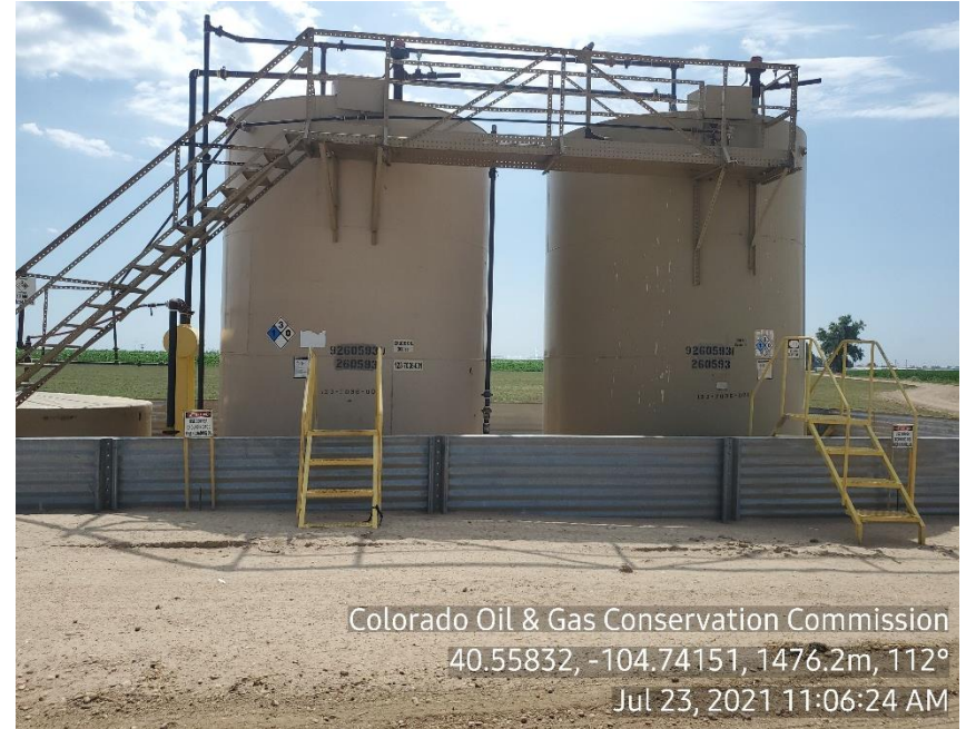
Photo 4: Tank Battery
