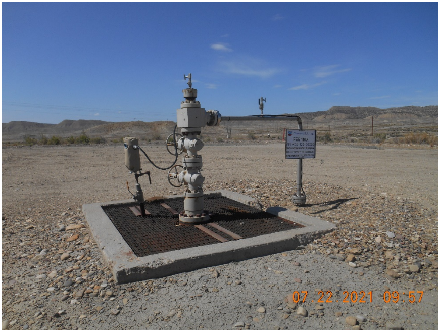
Injection wellhead.
