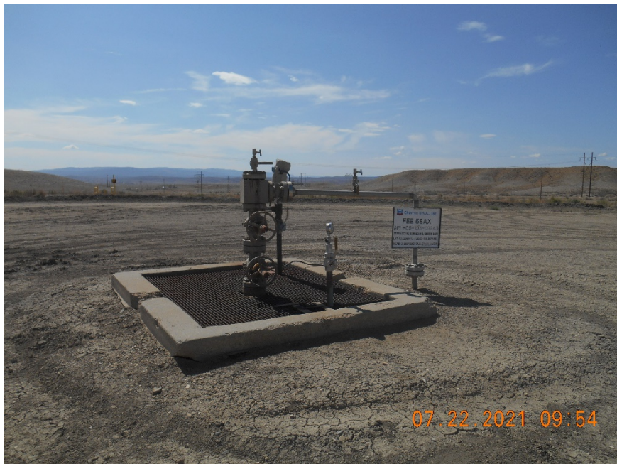
Injection wellhead.
