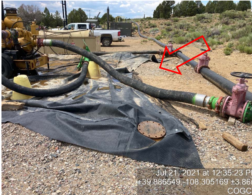
No berm on side of pump
