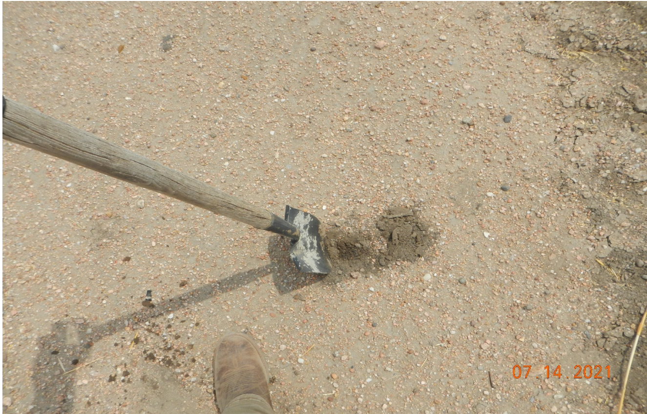
Photo 5. The soils throughout the location are compacted. The shovel could not penetrate through the soil.
