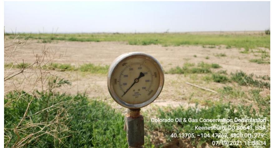
Photo 3 Tubing pressure gauge.
